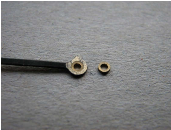
Bush in rod ready for soldering.
