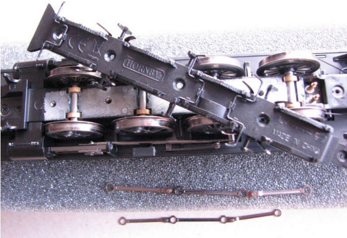
Keeper plate removed.
